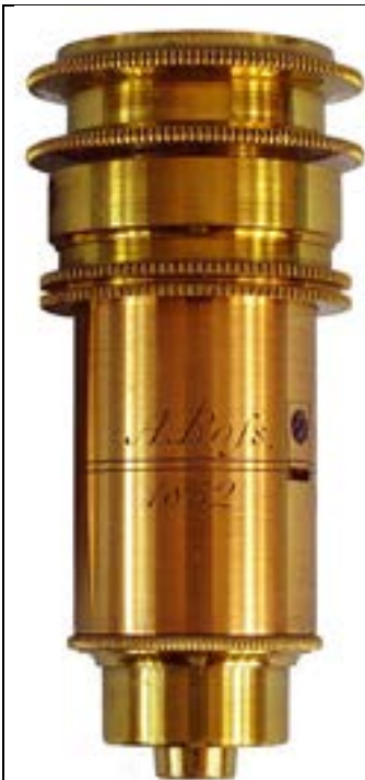
A. Rofs, 1852. Uncovered, Covered. \frac{1}{4} In. A. Rofs, London" on canister lid. With correction collar for variations in coverslip thickness, invented by Ross in 1837. 51mm.
