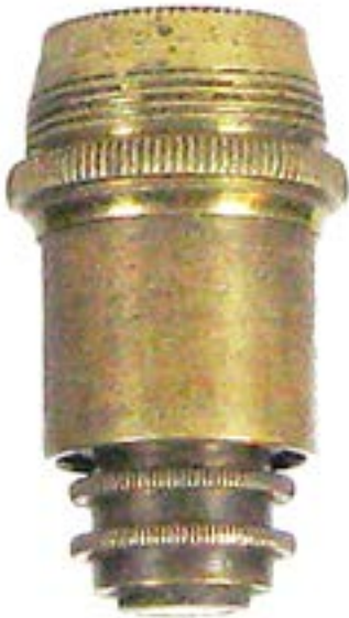
Three element, early achromatic objective by Andrew Pritchard. c1836. Pritchard (1804-1882) was one of the earliest established commercial providers of microscope slides in London, being in business from the mid 1820s until the late 1850s. 28mm.
