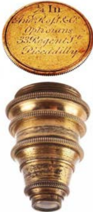
1/4 In, And r . Rofs & C o ., Opticians, 33 Regent S t ., Piccadilly" on canister lid. One of the first achromatic objectives, made between 1839 and 1843. One of the foremost microscope makers in London, Andrew Ross (1798-1859) began business in 1830 and collaborated with Joseph J. Lister (1786-1869) who perfected achromatic lenses. 26.7mm.
