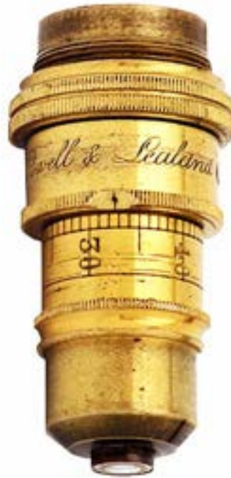
Powell & Lealand, N.A. 0.71. c1860. Correction collar. Hugh Powell (1799-1883) formed a partnership with his brother in law Peter H. Lealand in 1841. Hugh Powell, Andrew Ross, and James Smith produced the finest microscopes of the mid nineteenth century. 50mm.
