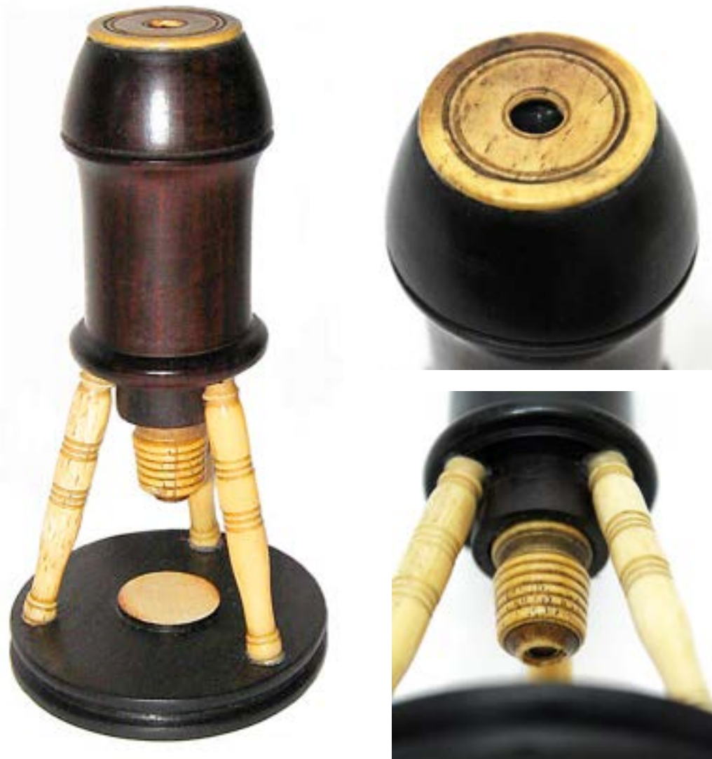
Compound Tripod Microscope, Second Half Seventeenth Century
