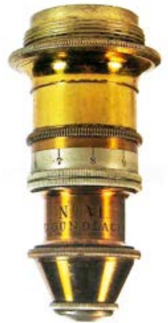
N° VI, E. Gundlach. \frac{1}{12} in" on lid. c1870. Correction collar. Ernst Gundlach (1834-1908) worked in Berlin from 1865 to 1871 before coming to America. He worked for Bausch & Lomb from 1876 to 1878 and operated the Gundlach Optical Company in Rochester from 1884 to 1895. 49mm.
