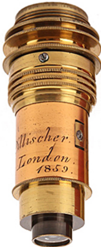
M. Pillischer, London, 1859, Uncovered, Covered. \frac{1}{2} inch. Early RMS thread. Moritz Pillischer made microscopes from about 1851 to 1887. 59mm.
