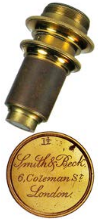
Unmarked pre-RMS objective. "1 1/2 Smith & Beck, 6 Colman St. London on canister lid. c1850. James Smith (d1870) produced some of the first achromatic microscopes with Joseph J. Lister. He took Richard Beck as partner in 1847 and the firm was known as Smith & Beck until 1857. 45mm.
